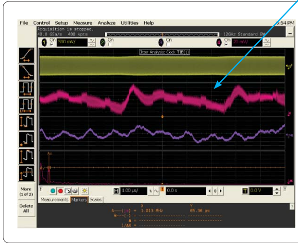
Figure 6. You can see a strong correlation between the clock jitter trend (purple) and the power waveform (pink).
